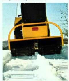
Note Alpine's single ski, its unique design always keeps you safely on course even on difficult side hills. Strengthened heavy duty metal plates absorb the sheek from jumps and bumps.
