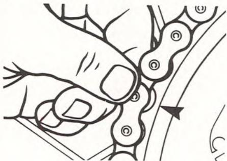
▼ **CAUTION:** A worn chain will cause severe sprocket damage.
