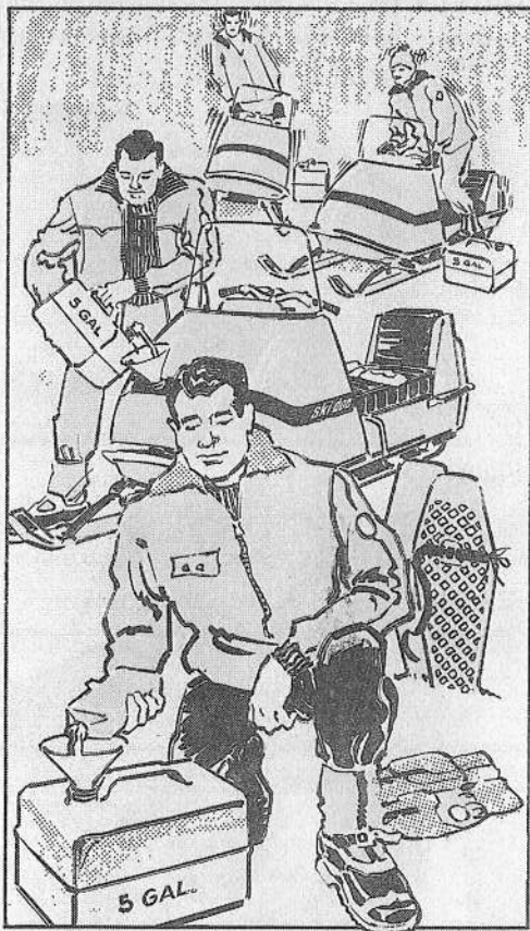
Fig. 26 shows the quantity of Ski-Doo oil required to mix, in a ratio of 20:1, a given quantity of gasoline.
