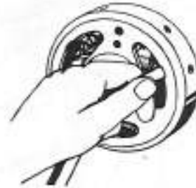
Checking the air gap
