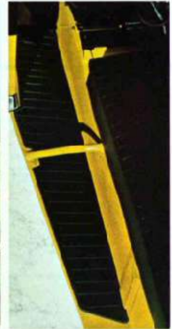
For greater safety, new running board mats prevent slipping when wet with snow.
