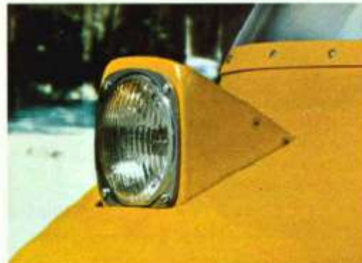
Mechanism on the dash swings up the newly-designed headlight for night SKI-DOOing.
