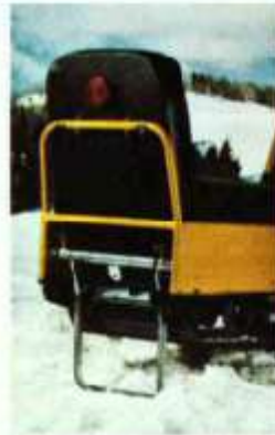
New combination rear bumper and kick-stand is heavy duty chrome. It swings down to lift track for faster warm-ups. Note, too, built-in positive trailer hitch!
