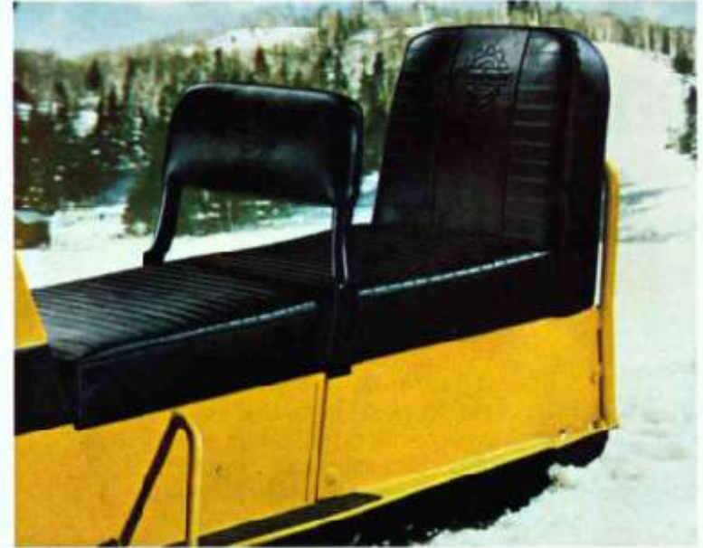
For greater comfort, seats have two layers of airfoam under a new stretch-free heavy-duty vinyl cover. New additional removable back rest is optional on all models.
