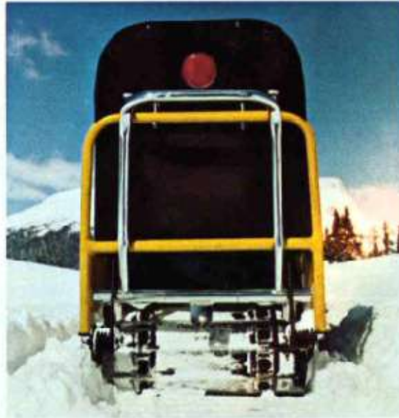
New combination rear bumper and kick-stand is heavy duty chrome. It swings down to lift track for faster warm-ups. Note, too, built-in positive trailer hitch!
